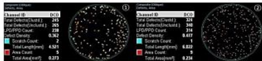
Defectivity mapping on new pad
